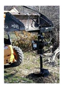
The 814H and 824H models clamp on to the bucket for easy on and off. Each unit slips on to the cutting edge of the bucket and has two turnbuckles and chains to secure it to the bucket.
