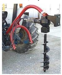
The models 614H and 624H three-point post hole diggers are designed for the operator without a front loader but likes the benefits that hydraulic operation. Both the 614H and 624H mount to tractors with cat. I/II hitches.
